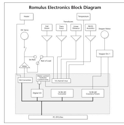
The ROMULUS material tester uses LabVIEW software and an IOtech DaqBoard/2000 as the heart of the data acquisition function as well as several control functions. The DaqBoard output controls a dc servomotor and heaters, motor control switches, and a stepper motor. Inputs include a number of transducers including temperature, linear distance, and force.
